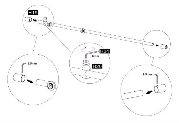
5 - Install the top rail with the wall brakets on the fixed panel H03 with the parts H21(X). -Mark the position of the wall brakets on the wall.
